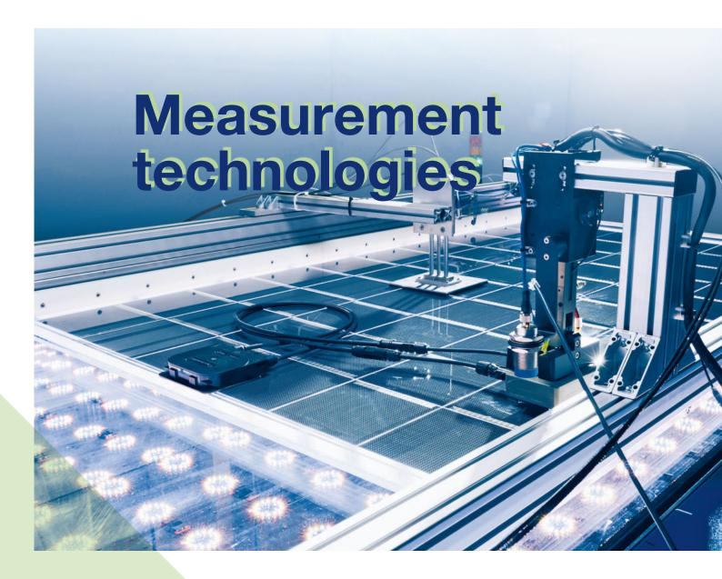
Wafer inspection systems, cell testers and module inspection systems detect quality defects and measure performance. Measurement technologies are indispensable in the production of efficient, high quality solar products.
