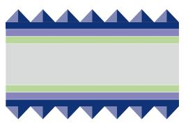
Transparent conductive oxide Doped amorphous silicon Intrinsic amorphous silicon
